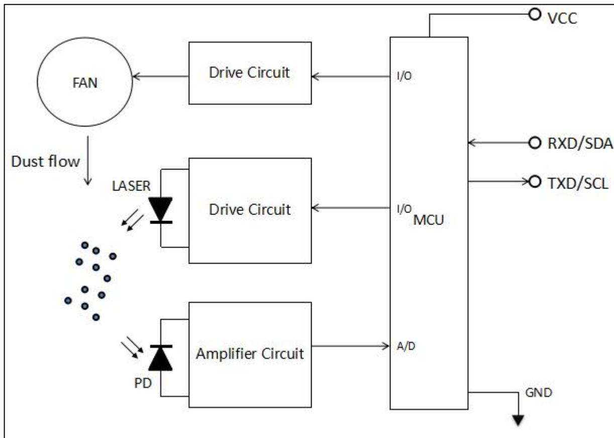
According to the above figure, The light source part of PM2012SE-B is composed of a laser tube and a driving circuit. The detection part of the sensor is composed of light sensitive part which receives reflected light and amplifying circuit. Data processing and communication output are completed by microprocessor.
