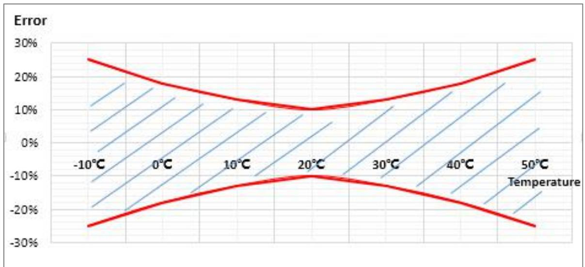
Particle measured error: under  $25 \pm 2^\circ\text{C}$ ,  $50 \pm 10\% \text{RH}$ ,  $0 \sim 1000 \mu\text{g}/\text{m}^3$ , consistency and accuracy of  $\text{PM}_{1.0}/\text{PM}_{2.5}$  is  $\pm 10\%$  reading or  $\pm 10 \mu\text{g}/\text{m}^3$ , use the biggest one (TSI-8530, Cigarette)
