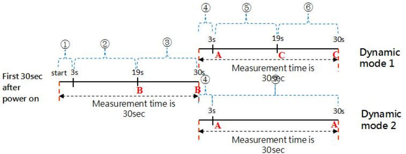
After sensors are in dynamic working mode, start measuring every 30s. The sensor starts the measurement for the first 3 seconds.
