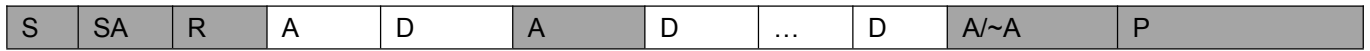
Picture 3: The general data format received from the slave device to the master device
